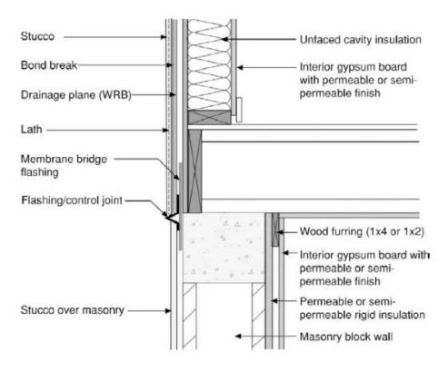
FIGURE 1403.9 FLASHING FOR DRAINED WALL ASSEMBLY OVER MASS WALL ASSEMBLY
