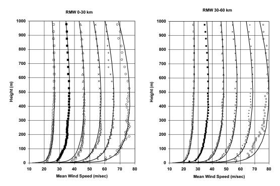
Figure 2-7. Modeled and observed hurricane mean vertical profiles of horizontal wind speed over the open ocean for a range of mean wind speeds
