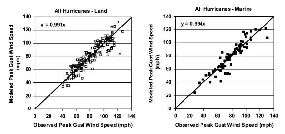
Figure 2-9. Example comparisons of modeled and observed maximum surface level peak gust wind speeds from landfalling hurricanes. Wind speeds measured on land are given for open terrain and wind speeds measured over water are given for marine terrain.
