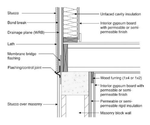
FIGURE R703.18 FLASHING FOR DRAINED WALL ASSEMBLY OVER MASS WALL ASSEMBLY
