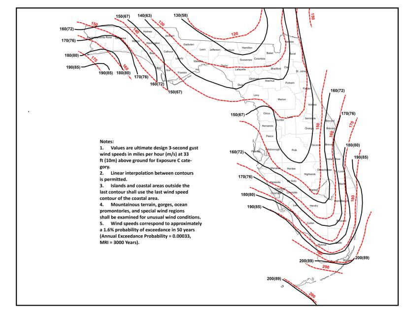
FIGURE 1609.3(3) (For Comparison Purposes Only – the 3,000-year return period map is not included in 6<sup>th</sup> Edition FBC) ULTIMATE DESIGN WIND SPEEDS, *Vuιτ*, FOR RISK CATEGORY IV BUILDINGS AND OTHER STRUCTURES (red dashed lines are existing ASCE 7-10 contours) Site Specific Wind Hazards & Enhanced Design Wind Speeds
