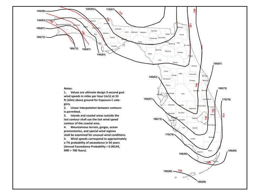
FIGURE R301.2(4) 6<sup>th</sup> and 7<sup>th</sup> EDITION FBC (Residential) ULTIMATE DESIGN WIND SPEEDS V<sub>ult</sub> (red dashed lines are existing FBC contours)
