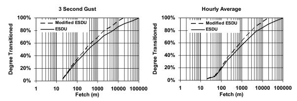
Figure 2-8. ESDU and modified ESDU wind speed transition functions at 10 m elevation.
